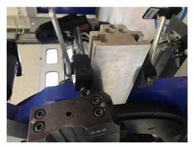
THE SETTING OF THE TOOLOBOXES, TOOLS, AND SUBSEQUENT SETTING OF THE CUT & BEVEL TOOL ENGAGEMENT TO THE PIPE WALL IS CRITICAL TO ACHIEVE CONSISTENT RESULTS, OPTIMUM PERFORMANCE & CUTTING SPEEDS, COMBINED WITH DESIRED TOOL LIFE
