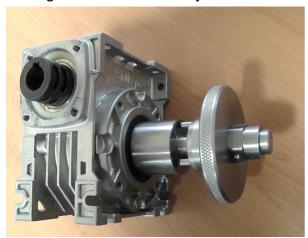
X AXIS travel can be controlled manually or with smooth, consistent power feed from an infinitely variable & reversible pneumatic or hydraulic drive system.
