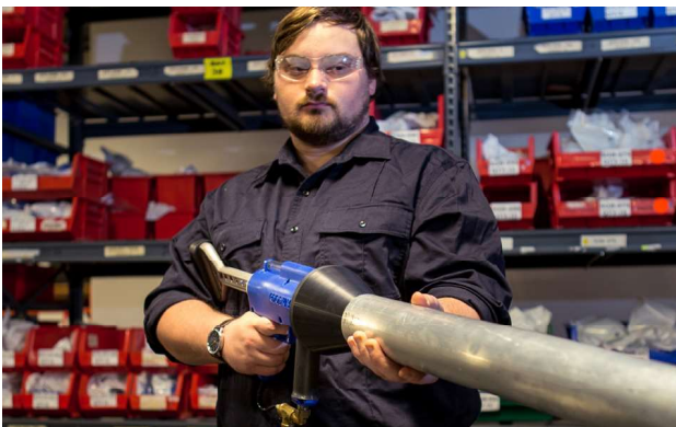
PNEUMATIC HOSE/TUBE CLEANING GUN FOR TUBES 50 TO 114 MM
