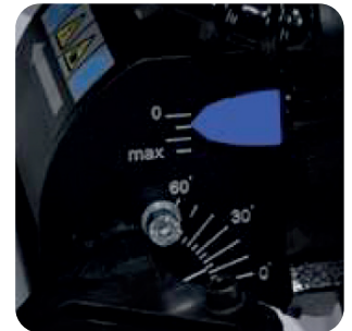
Continuous angle adjustment from 0 to 60 degrees.
