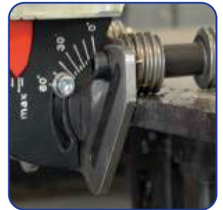
Continuous angle adjustment from 0 to 60 degrees.
