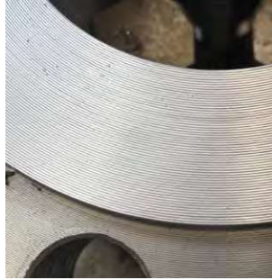
Single line gramophone groove (50 grooves per 1 inch)
