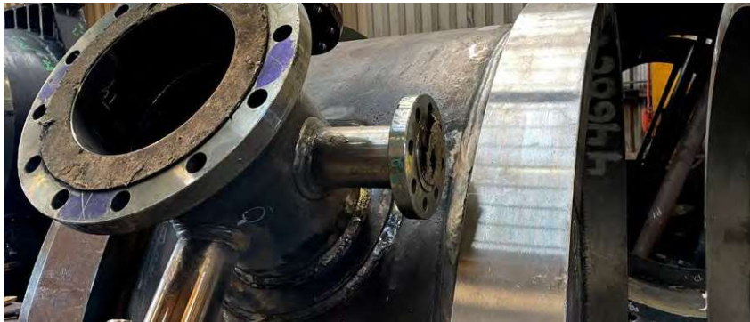
Example of really tight flange – NBFF is the only tool suitable here.
