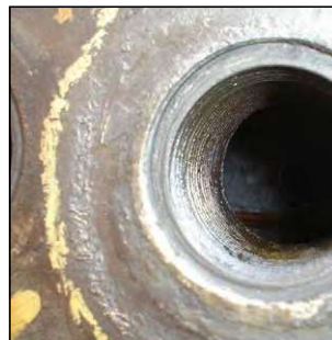
Plug hole before re machining the gasket seat
