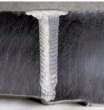
Narrow Gap Bevel Geometry shown on 25 mm [1"] wall pipe
