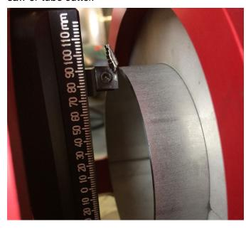
Tube with small diameters <25.4 mm are particularly concerned by the facing process. They are often cut with tube cutters or abrasive cutting machines. Generally speaking, tube must be faced before welding in order to obtain quality welds.
